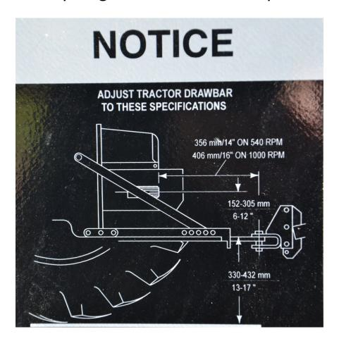
The distance from the end of the PTO shaft to the pin on the pull bar of the tractor must be 14" as illustrated above. Otherwise, damage will occur to the baler.
