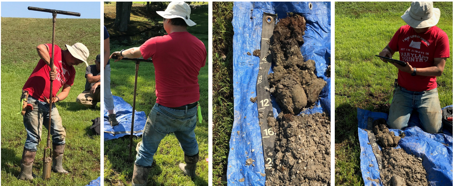
NRCS Regional Soil Scientist, Jason Martin, analyzes soil borings with district staff for an upcoming pond design project.
